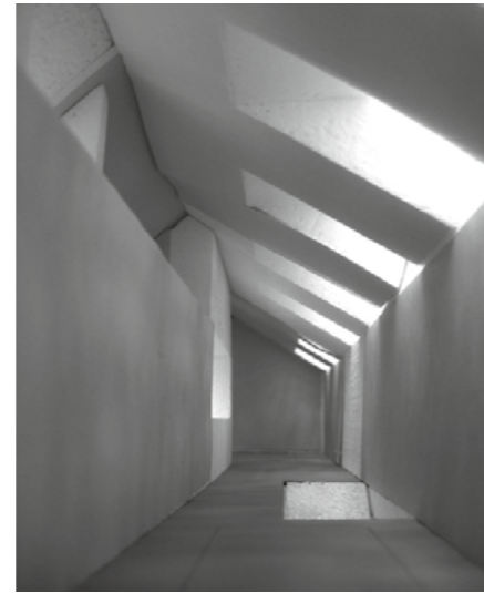
Daylight simulation with physical model.
