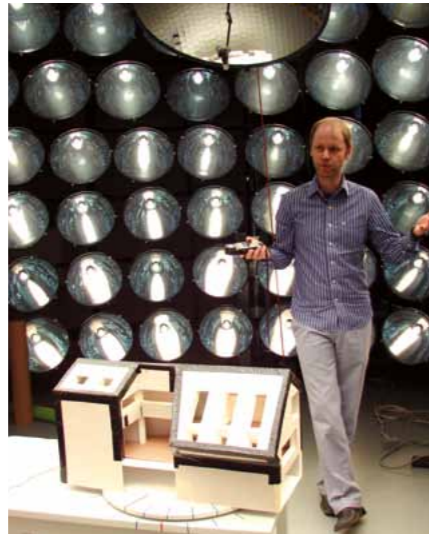
Daylight simulation with physical model in daylight laboratory performed by Arch. DI Gregor Radinger, Donau-Universität Krems.
