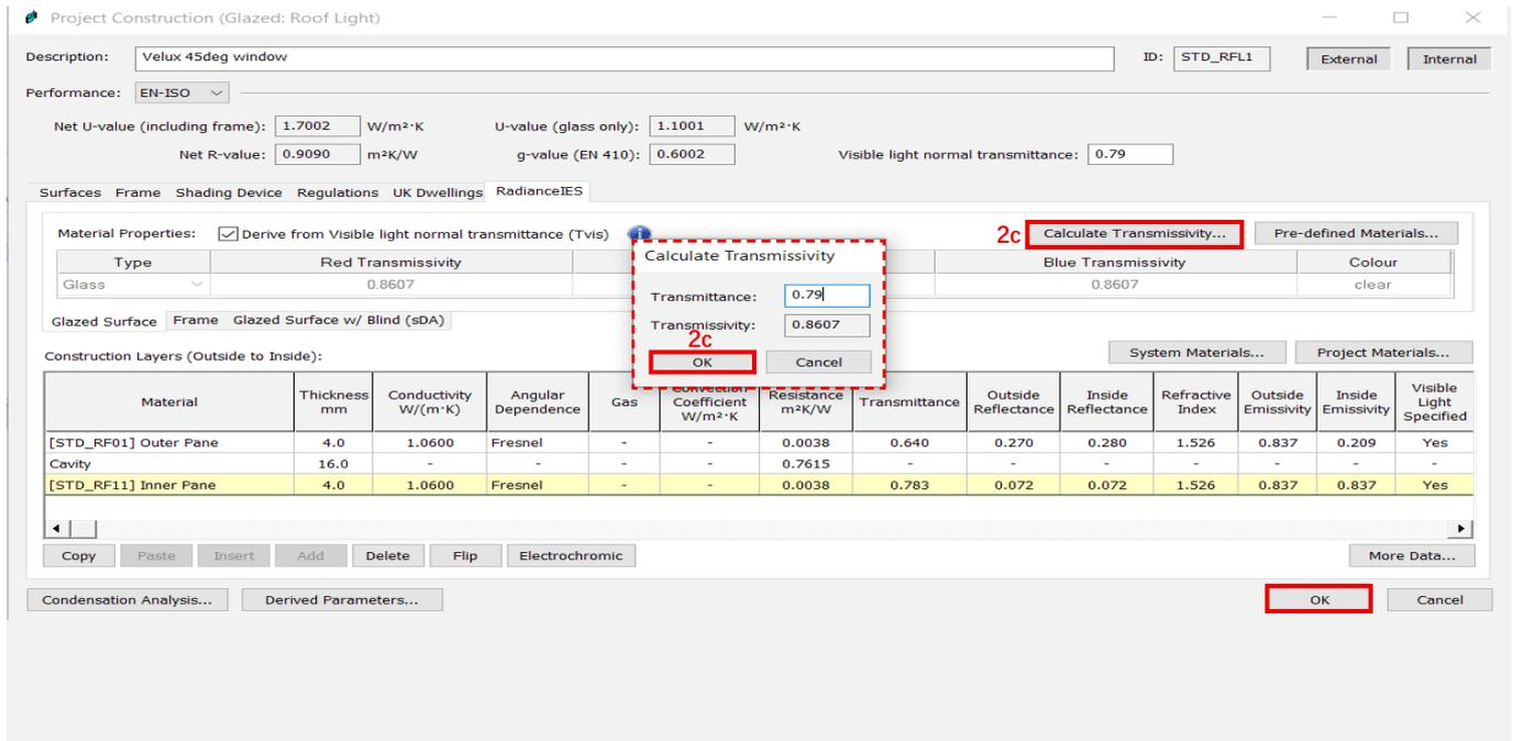
Figure 11, APcdb glazed construction window RadianceIES tab - Frame sub-tab
