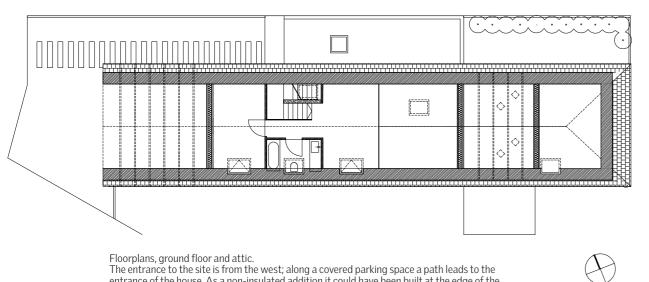
Floorplans, ground floor and attic. The entrance to the site is from the west; along a covered parking space a path leads to the entrance of the house. As a non-insulated addition it could have been built at the edge of the site. Behind the open living area is the master bedroom with en-suite bathroom. An open space on the east side of the attic is usually filled with toys.
