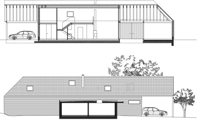
Longitudal sections through the house. A clear order of the spaces in the house: parking lot, bedrooms, kitchen with an open space above are stacked next to the double-height living area and veranda. The second section shows the entrance area, lightened through a VELUX flat roof window and the heating room. Except for the roof windows and one bathroom window this facade is entirely closed.
