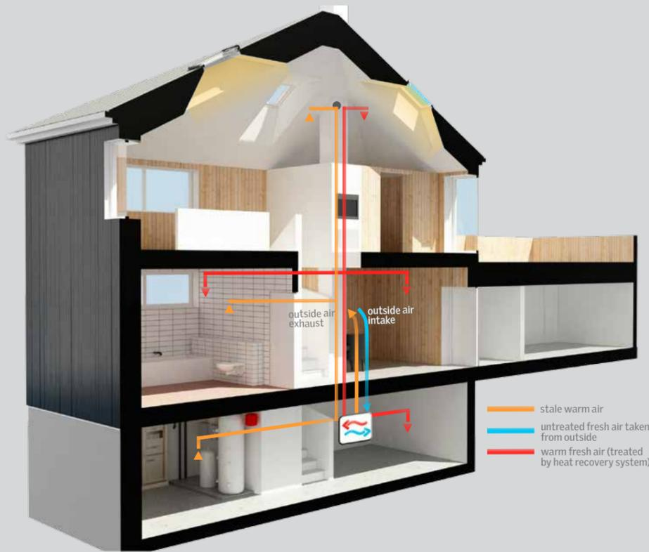
**In the winter**, mechanical ventilation will take fresh outdoor air into the house and pre-heat it in a heat exchanger (using a heat recovery system), thereby reducing the energy required for warming cold air.
