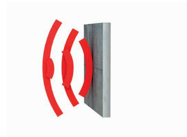
Enclosure in metal. Loss: 90 to 100%
