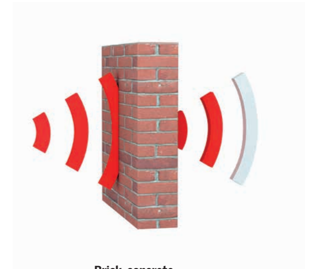
Brick, concrete. Loss: 20 to 40%
